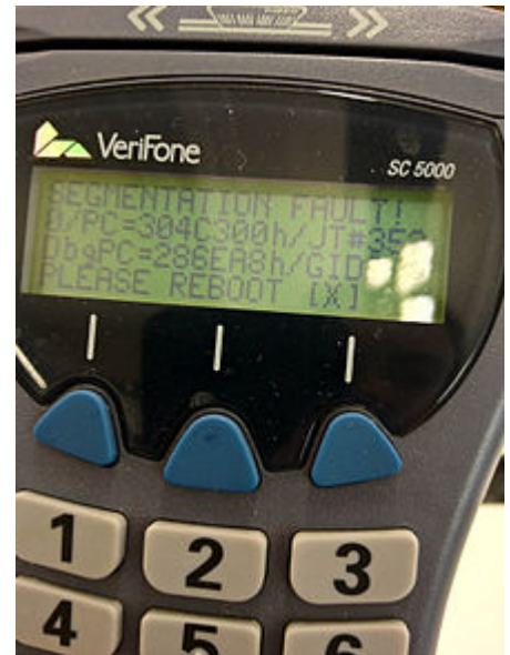
Segmentation fault on an EMV keypad
